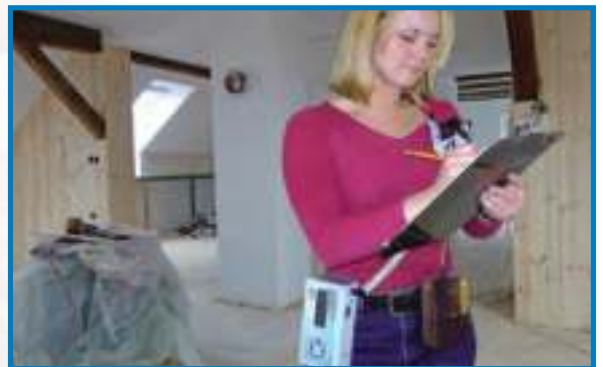
Attach to a pump to monitor dust levels in real time while collecting a gravimetric sample. SKC recommends using the AirChek 52/Sidekick pump. See pages 24-25.
