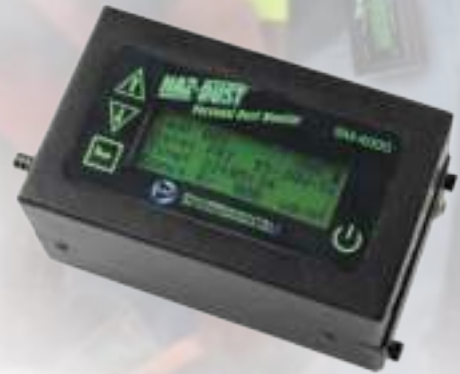
Clip the sensor with GS-3 Cyclone to a worker's collar in the breathing zone.
