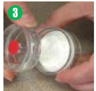
3 Complete cassette assembly. After sampling, remove Accu-CAP from cassette and weigh.
