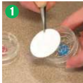
1 Prepare SKC 2-piece cassette with support pad.
