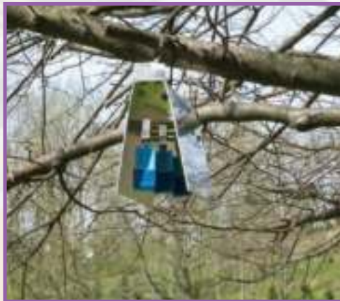
Outdoor sampling shelter protects multiple samplers.
