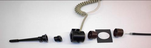
Figure 3.3. Component identifications from left to right: SKC GS-Cyclone for Respirable sampling, GSA-202 adapter, sensor head, disassembled filter cassette, filter, and air intake tubing.
