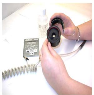
Figure 5-3. Removing the sensor cover.
