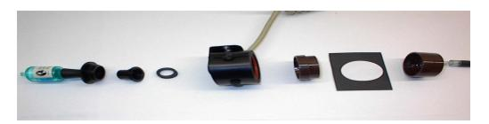
Figure 3.7b. Zeroing filter (p/n ZA-202A) being attached to the Inhalable sampling inlet.
