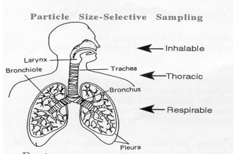
Figure 1-4. Diagram showing breathing zones of Inhalable, Thoracic, and Respirable dust particles.
