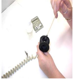
Figure 5-6. Sensor head being cleaned with cotton swab.
