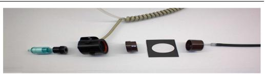
Figure 3.7c. Zeroing filter (p/n ZF-102) being attached to GSAS-202 GS-Cyclone adapter.
