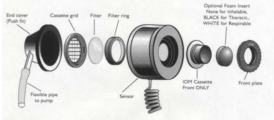
Figure 3-5. Disassembled IOM Sampling Adapter. SKC catalog number 225-70.
