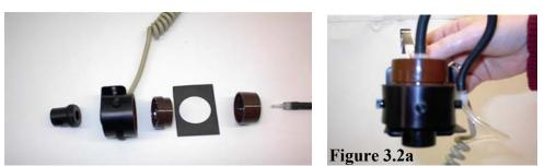
Figure 3-2 and 3-2a. Thoracic Inlet, sensor head, disassembled filter cassette, 37 mm filter, and air intake tubing. Optical sensor mounted on lapel bracket.
