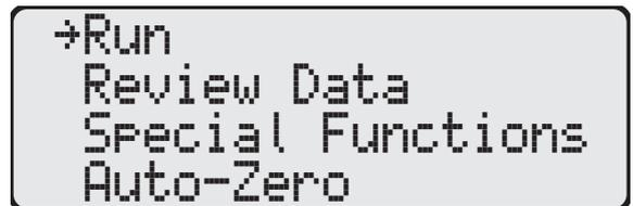
On the Run menu screen select the Run - Continue option to begin sampling with the alarm function disabled, retain the existing data and store the new data in the next available memory location.
