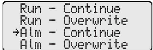
Alternatively select the Alm - Overwrite option to begin sampling with the alarm function enabled, delete the existing data and store the new data in memory location 001.
