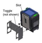
Rotate the holder 90 degrees so that the toggle catches securely inside either side of the slot and the bottom plate of the holder is parallel with the bottom of the pump.
