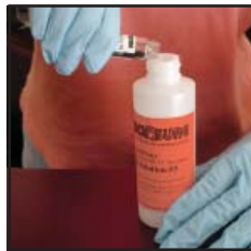
Pour one vial of Disclosing Powder #1 into Developing Solution #3 spray bottle.
