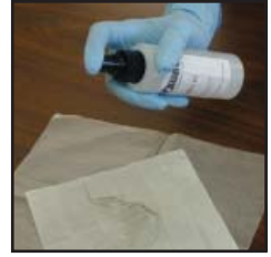
Aim at soiled wipe and depress nozzle 3 times.
