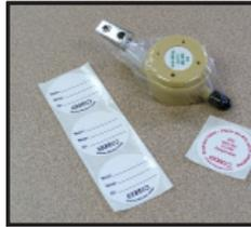
2. Write sample ID on sampling label. Adhere sampling label to **bottom** of base plate.
