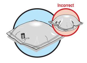
Secure polypropylene valve when opening/closing by holding side stem while turning entire upper portion of fitting one revolution.
