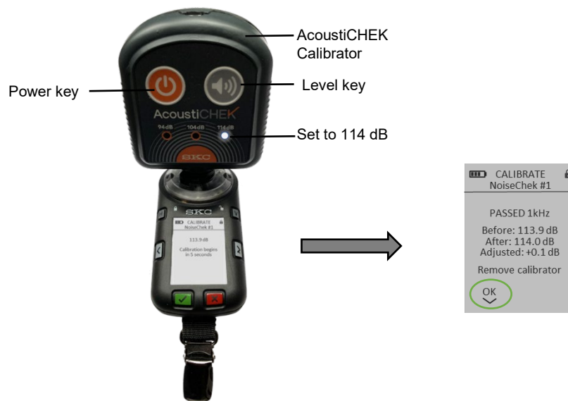
Figure 3. Calibration Train and Display
