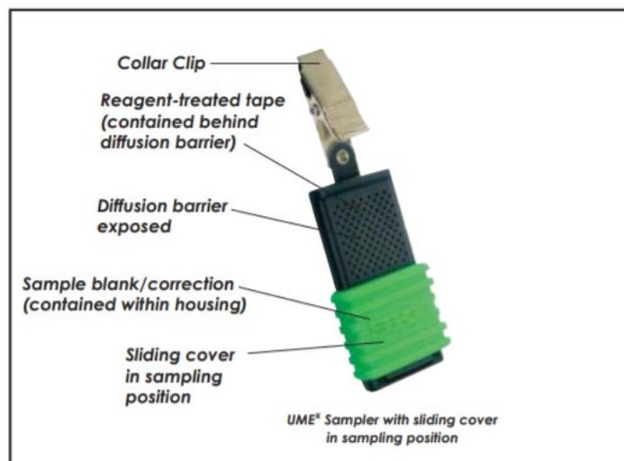
After sampling, slide the sampler cover to the "off" position (cover diffusion holes) to stop sampling. Unclip the sampler and record the sample stop time on the label on the back of the sampler. Place the sampler into the resealable pouch immediately after sampling. Seal the pouch.
