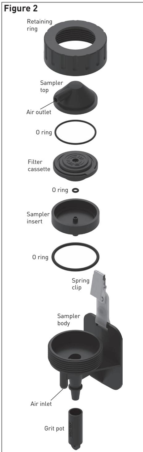
the cassette. Fit the retaining ring over the sampler top and screw down firmly to secure the cassette within the sampler and seal the cassette inlet and outlet.
