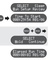
The pump will run for the programmed sample runtime and at the end of this the pump will automatically stop, and the repeat delay countdown time will be displayed. The repeat counter will increment.
