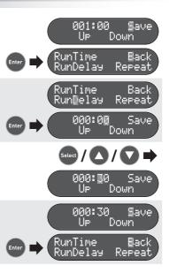
To program repeat sample run and delay times, on the 'RunTime' menu screen cycle to the 'Repeat' option, and press at to display the 'Set Repeat' menu screen.
