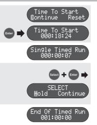
Press the and mean keys simultaneously to return to the 'SELECT' main menu screen.
