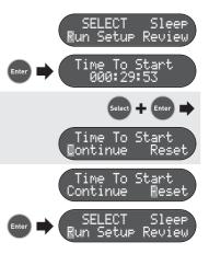
Alternatively, on the reset screen cycle to the 'Continue' option and press at to return to the start delay countdown.
