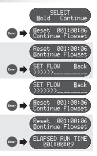
To complete the manual sample run at the end of the required sample time, on the Hold menu screen cycle to the 'Reset' option and press . The display will return to the 'SELECT' main menu screen.
