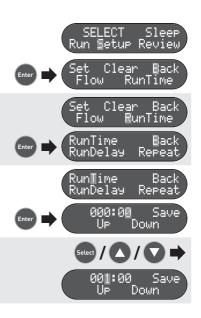
Cycle to the 'Save' option and press en to save the sample runtime and return to the 'RunTime' menu screen.
