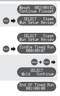
Press the and and keys simultaneously to return to the 'SELECT' main menu screen.
